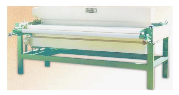
The principle of Dedusting machine is designed to carry leather into machine for dust removing by conveyor using. Through 3 sets wind mouthpieces of 0.1 mm clearance, the machine can clean and remove leather dust completely by blower and the dust collection box. Also the operation speed can be adjusted as control of continuous variable transmission.
